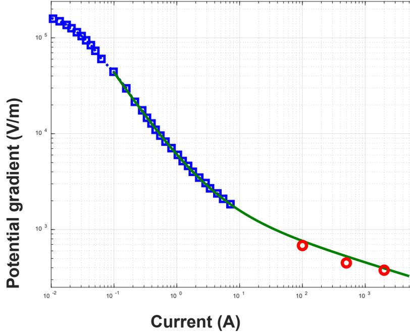
Fig. 3. Electric field versus current in arc channel
