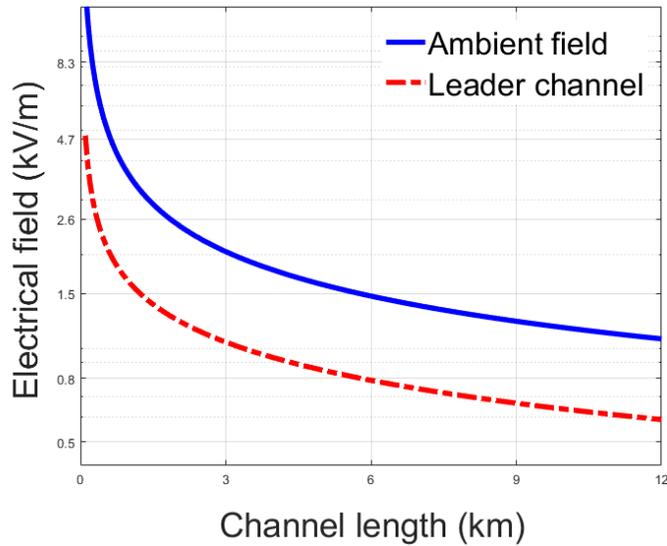
199 Fig. 6. variations of ambient electric field of the leader-streamer system and electric field of the leader
