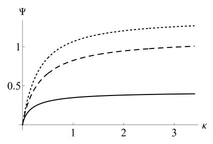
**Figure 11.** Solitary wave amplitude in the homogeneous trapped distribution, non-drifting and non-oscillating case as a function of  $\kappa$  and different  $\alpha$ 's, from Eq. (36). Upper, dotted line:  $\alpha = 0.0$ ; mid, dashed:  $\alpha = 0.5$ ; Lower, solid:  $\alpha = 1.5$ .
