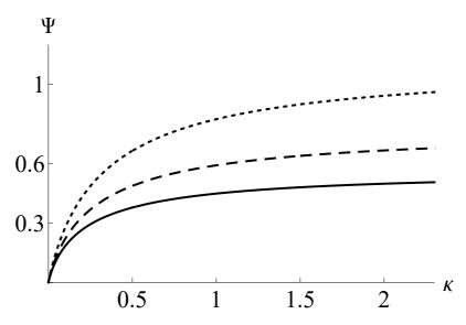
Figure 12. Wave amplitude in the homogeneous trapped distribution, non-drifting and oscillating case as a function of  $\kappa$  and different wavenumbers, for  $\alpha = 1.5$ , from Eq. (35). Lower, solid:  $k_0 = 1.0$ ; mid, dashed:  $k_0 = 1.5$ ; upper, dotted line:  $k_0 = 2.0$ .
