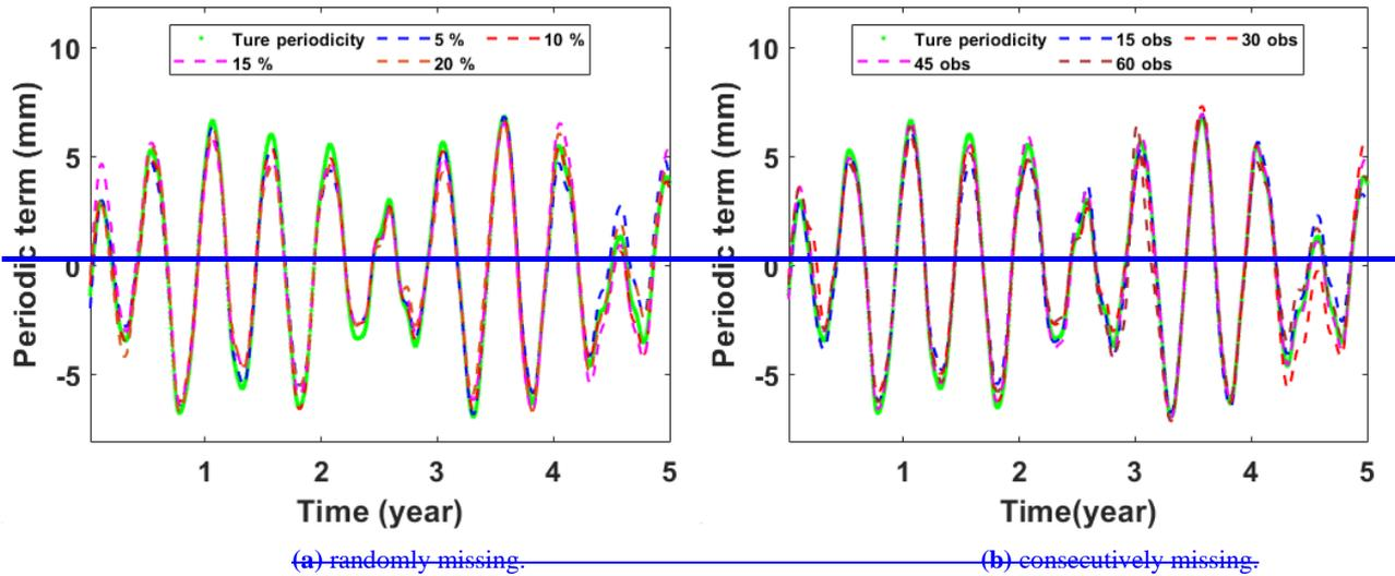
**Figure 5: The obtained periodic signal and the real periodic signal of (a) randomly missing and (b) consecutively missing.**
