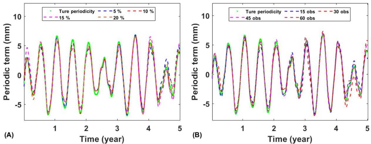
230 Figure 4: The obtained periodic signal and the real periodic signal of (A) randomly missing and (B) consecutively missing.
