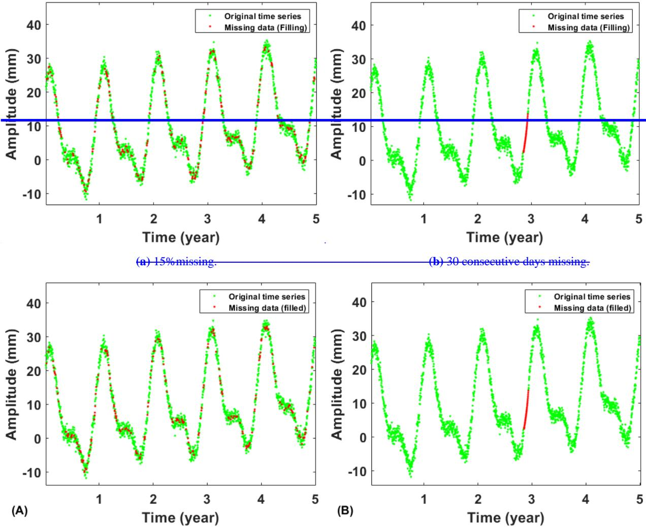
Figure 2: Data filling of (a)(A) random missing 15% and (b)(B) consecutive missing 30 days.
