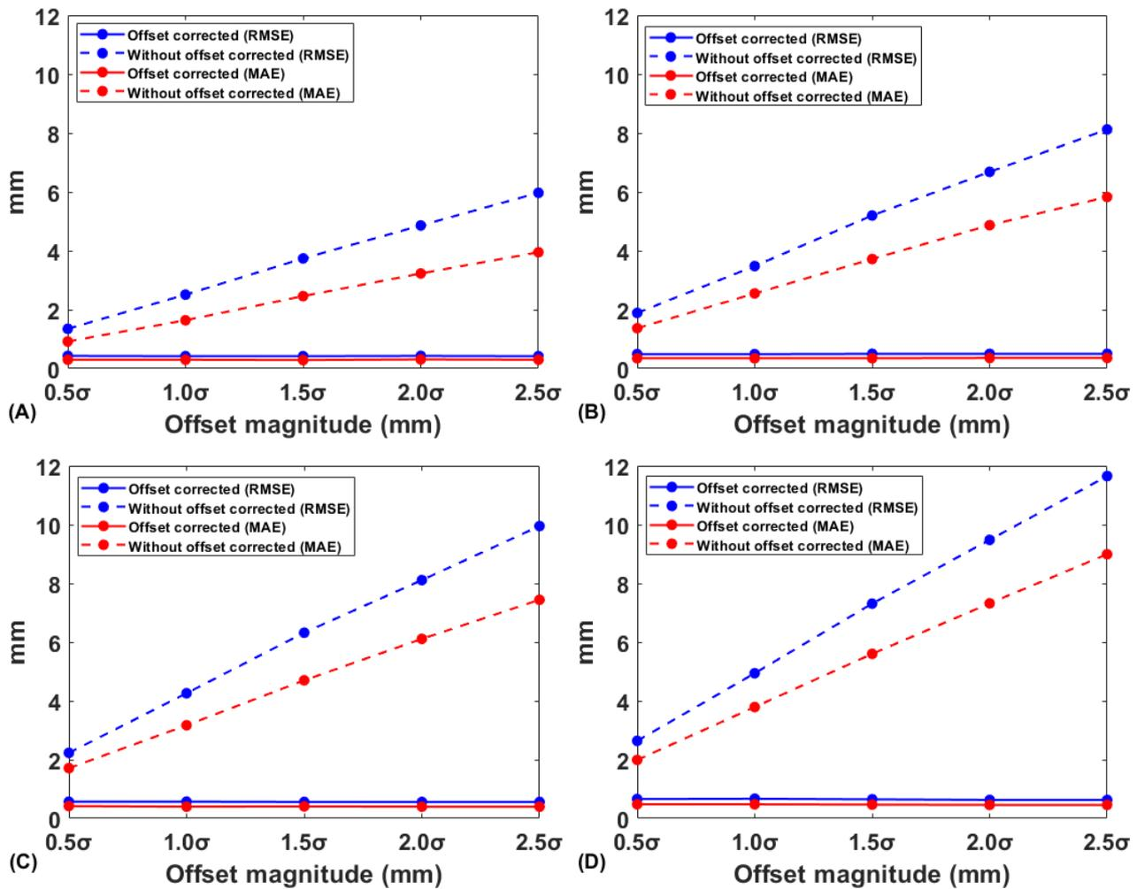
Figure 6: Periodic signal RMSE and MAE with and without offset correction of different number and magnitude offsets (a)(A) 2 offsets, (b)(B) 4 offsets, (c)(C) 6 offsets and (d)(D) 8 offsets.
