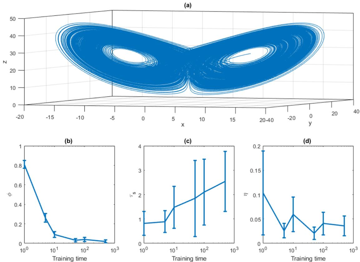
**Figure 1.** (a) Lorenz 1963 attractor obtained with an Euler scheme with  $dt = 0.001$ ,  $\sigma = 10$ ,  $r = 28$  and  $b = 8/3$ . Panels (b)–(d) show the performance indicator as a function of the training time. (b) The rejection rate  $\phi$  of the invariant density test for the  $x$  variable; (c) the first time  $t$  such that  $APE > 1$ ; (d) the initial error  $\eta$ . The error bar represents the average and the standard deviation of the mean over 100 realizations.
