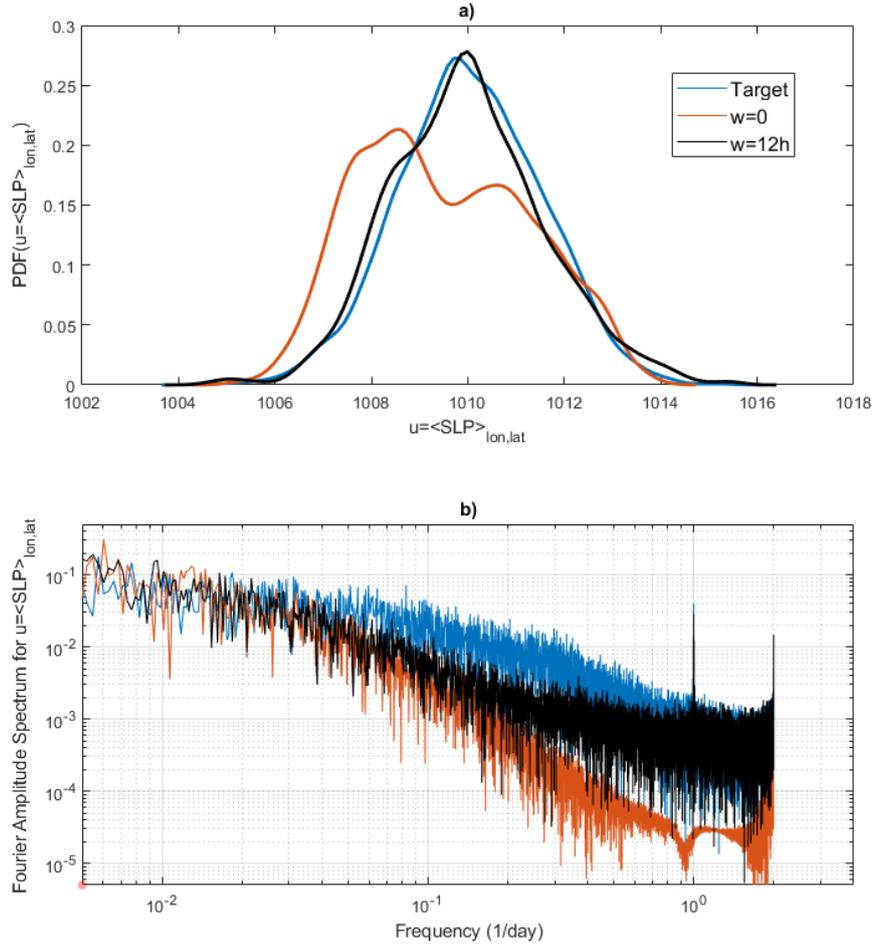
**Figure 10.** a) probability density function and b) Fourier power spectra for  $u(t) \equiv \langle SLP(t) \rangle_{lon,lat}$  for the target NCEPv2 SLP data (blue), an ESN with  $c = 4$  and  $w = 0$  h (red), and an ESN with  $c = 4$  and  $w = 12$  h (black).
