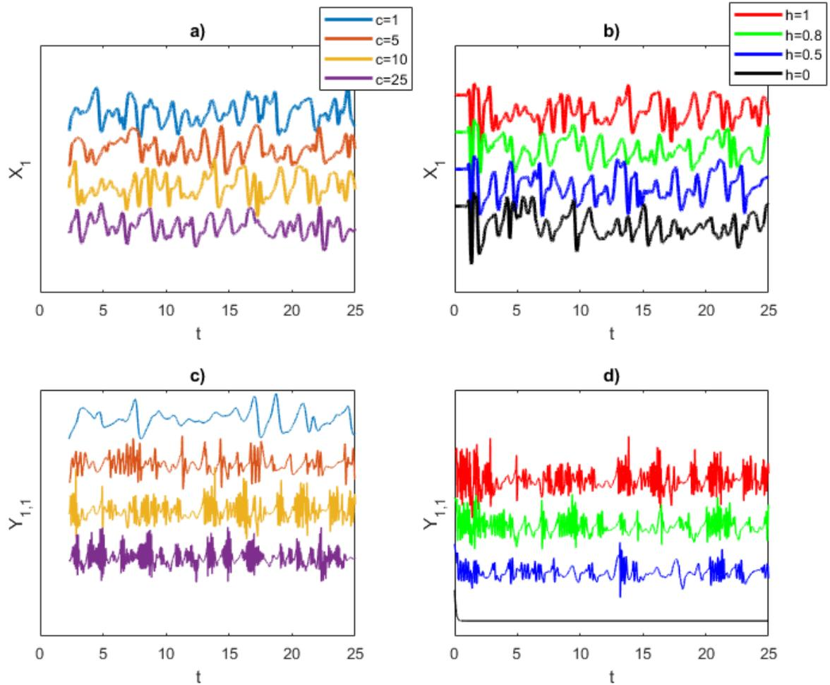
**Figure 6.** Lorenz 1996 simulations for the large-scale variable  $X_1$  (a,b) and small-scale variable  $Y_{1,1}$  (c,d). Panels (a,c) show simulations varying  $c$  at fixed  $h = 1$ . The larger  $c$ , the more intermittent the behavior of the fast scales. Panels (b,d) show simulations varying the coupling  $h$  for fixed  $c = 10$ . When  $h = 0$ , there is no small-scale dynamics.  $y$ -axes are in arbitrary units, time-series are shifted for better visibility.
