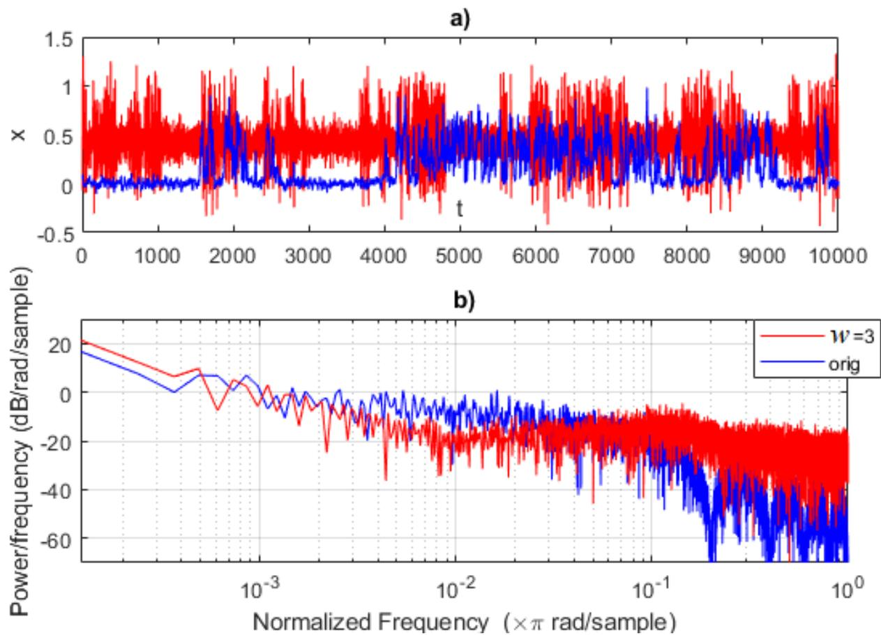
**Figure 5.** Pomeau-Manneville ESN simulation (red) showing an intermittent behavior and compared to the target trajectory (blue). The ESN trajectory is obtained after training the ESN for  $10^5$  time-steps using the moving average time series with  $w = 3$ . It consists of  $10^4$  time steps. Cases  $w = 0$  are not shown as trajectories always diverge. Evolution of trajectories in time (a) and Fourier power spectra (b).
