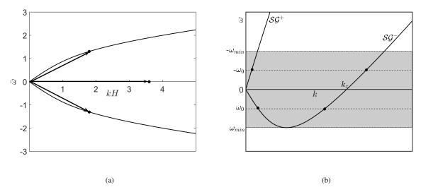
Figure 2. (a) A Bragg triad in the absence of mean velocity. Wavenumber k has been nondimensionalised by 1/H ( $H \equiv$  flow depth), while frequency  $\omega$  by  $\sqrt{g/H}$  i.e.  $\omega^* \equiv \omega/\sqrt{g/H}$ . (b) Bragg triads in the presence of 'Couette-type' mean velocity with  $Fr \equiv U/(\sqrt{gH}) = 0.7$ . In the shaded region, three Bragg triads can exist for a given k. For labels, see text.
