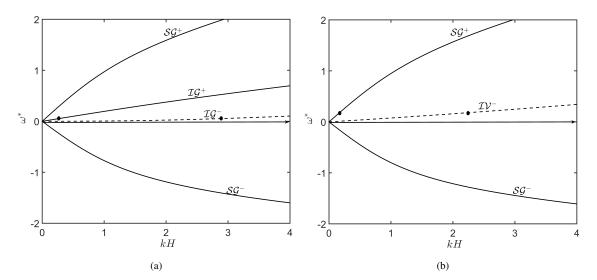
Figure 4. (a) Dispersion curves for a uniform current.  $U_u^* = U_l^* = U_b^* = 0.1, h_u/h_l = 1/3, \rho_u/\rho_l = 0.95$ . (b) Dispersion curves for shear in bottom layer and single density fluid.  $U_u^* = U_l^* = 0.1, U_b^* = 0, h_u/h_l = 1/3, \rho_u = \rho_l$ . Dashed curves have negative energy. U has been non-dimensionalised with  $\sqrt{gH}$ , where  $H = h_u + h_l$
