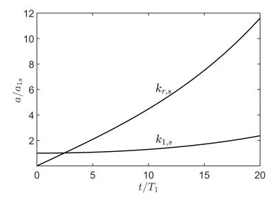
Figure 3. Growth of amplitudes of a wave on  $\mathcal{SG}^-$  branch which resonates a wave on the same branch. Relevant parameters are-  $k_iH=0.06, k_rH=3.13, k_bH=3.19, \omega_i/\sqrt{g/H}=-0.0213, \omega_i/\sqrt{g/H}=0.0213, U/\sqrt{gH}=0.70, N=2048, M=2, a_{1s}/H=2.5\times10^{-5}, a_b/H=0.025, T_i/\Delta T=1024.$
