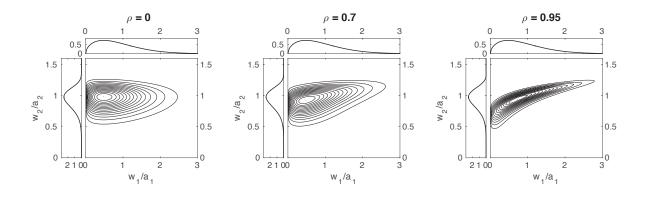
Figure 4. As in Figure 1 for the bivariate Weibull distribution with  $(a_1, b_1, a_2, b_2) = (4, 1.5, 5, 7)$  and  $\rho = 0, 0.7$ , and 0.95 and the speeds  $w_1, w_2$  scaled respectively by the Weibull scale parameters  $a_1, a_2$ .
