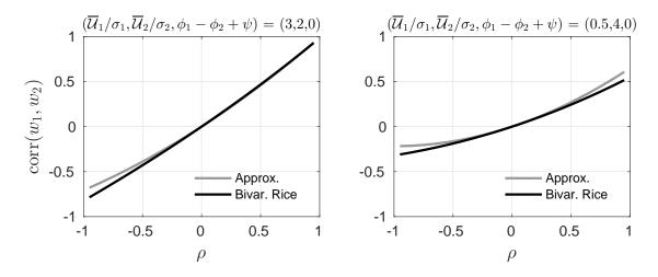
Figure 2. Comparison of the correlation coefficient  $corr(w_1, w_2)$  for bivariate Rice distributed variables (Eq. 38) with the approximate expression Eq. (40) for the parameter values  $(\overline{U}_1/\sigma_1, \overline{U}_2/\sigma_2, \phi_1 - \phi_2 + \psi) = (3, 2, 0)$  and (0.5,4,0).
