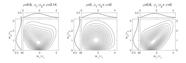
Figure 3. As in Figure 1 for the bivariate Rice distribution with  $(\overline{U}_1, \sigma_1, \overline{U}_2, \sigma_2) = (6, 4, 2, 5)$  and  $(\rho, \phi_1 - \phi_2 + \psi) = (0.8, \pi), (0, 0)$ , and (0.8, 0).
