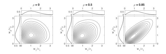
Figure 1. Example bivariate Rayleigh distributions  $p(w_1, w_2)$  for  $\rho = 0, 0.5$ , and 0.85, with  $w_1$  and  $w_2$  scaled respectively by  $\sigma_1$  and  $\sigma_2$ . The upper and left subpanels show the marginal distributions of  $w_1$  and  $w_2$  respectively. These marginal distributions are the same for all three panels.
