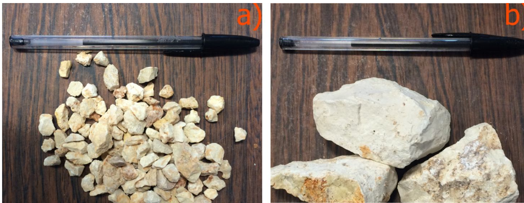
538 Figure 2. Samples of the materials used for the experiments with different average grain sizes d_p . a) d_p = 9.2 mm b) d_p = 41.6 539 mm.
