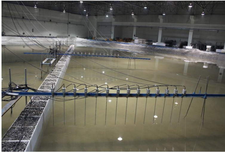
Photo 1. Experimental facility and wave gauge array.
