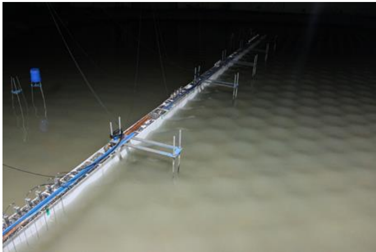
Photo 2. Wave pattern in front of a vertical wall ( \theta_0 = 30^\circ ).
