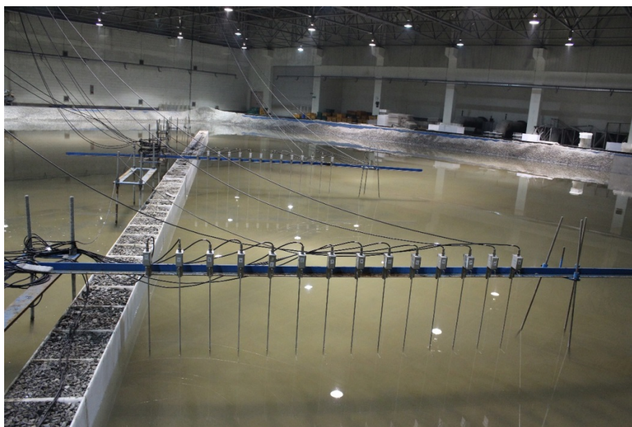
Photo 1. Experimental facility and wave gauge array.
