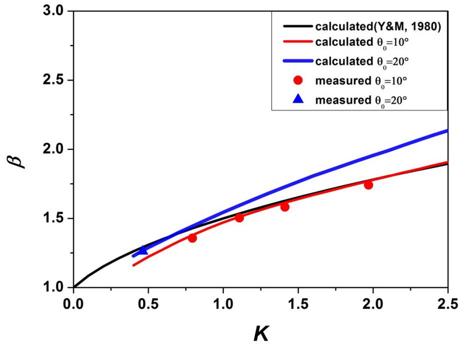
Figure 27. Comparison of calculated and measured  $\beta$  as a function of nonlinear parameter  $K$ . Black solid curve represents the calculated value using Yue and Mei (1980), red and blue solid curves denote the calculated values for  $\theta_0 = 10^\circ$  and  $20^\circ$ , respectively. Symbols are measured data.
