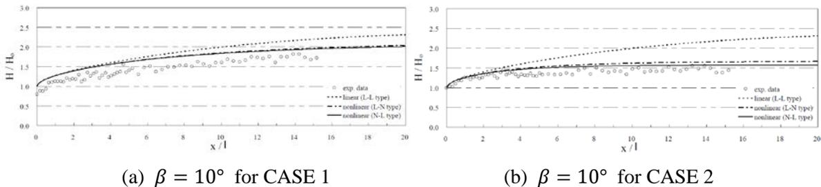
Figure 1. Relative wave height along the front wall of CASE 1 and CASE 2 (Lee and Kim, 2007)
