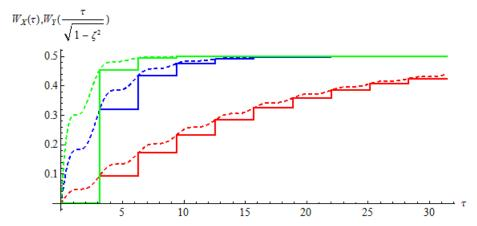
Figure 4: Dissipated energy of vibrations for fragmented media (solid line) and equivalent Kelvin-Voigt model (dashed line) for  $\alpha = 0.9$  (red),  $\alpha = 0.6$  (blue),  $\alpha = 0.3$  (green) and initial conditions  $X_0 = 0.0$  and  $V_0 = 1.0$ .
