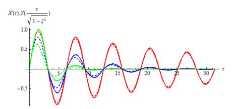
Figure 3: Vibrations for fragmented media (solid lines) and equivalent Kelvin-Voigt model (dashed lines) for  $\alpha = 0.9$  (red),  $\alpha = 0.6$  (blue),  $\alpha = 0.3$  (green) and initial conditions  $X_0 = 0.0$  and  $V_0 = 1.0$ .
