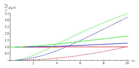
Figure 5: Velocity characteristics of a p-wave propagating in fragmented media: phase velocity (solid line) and coefficient of absorption (dashed line) for  $\alpha = 0.9$  (red),  $\alpha = 0.6$  (blue),  $\alpha = 0.3$  (green).
