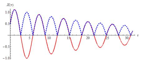
Figure 1: Vibrations for fragmented media (red solid line) and impact oscillator (blue dashed line) for absolute values of  $\alpha = 0.9$  and initial conditions  $X_0 = 0.5$  and  $V_0 = 1.0$ .
