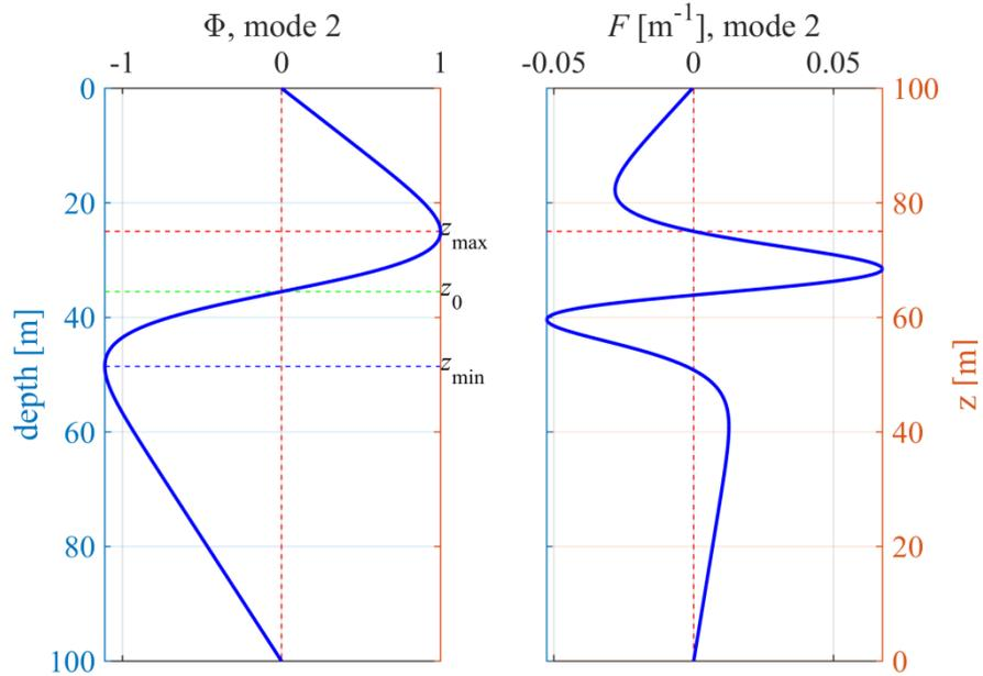
5 Figure 4: The vertical structure of the mode function  $\Phi(z)$  defined in Eq. (2) (left) and its nonlinear correction  $F(z)$  defined by Eq. (5) (right) for internal solitary waves of the second mode for stratification presented in Fig. 3.
