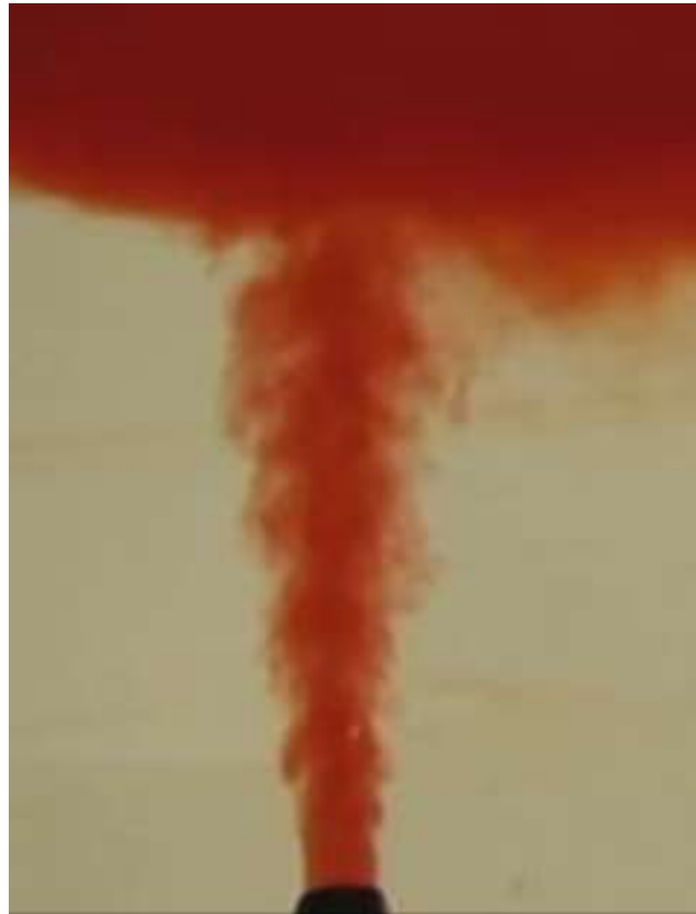
Figure 16: A snapshot from a movie (Carrozo et al., 2014, Supplementary Material S3), recording an experiment simulating a volcanic vent in a stratified water tank.
