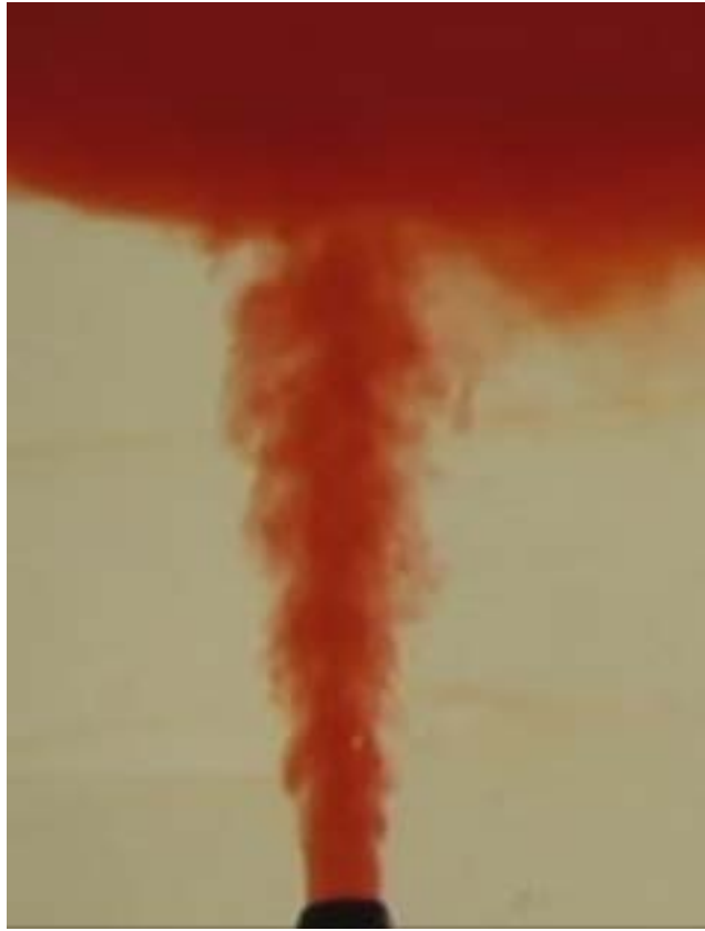
Figure 16: A snapshot from a movie (Carazzo et al., 2014, Supplementary Material S3), recording an experiment simulating a volcanic vent in a stratified water tank.
