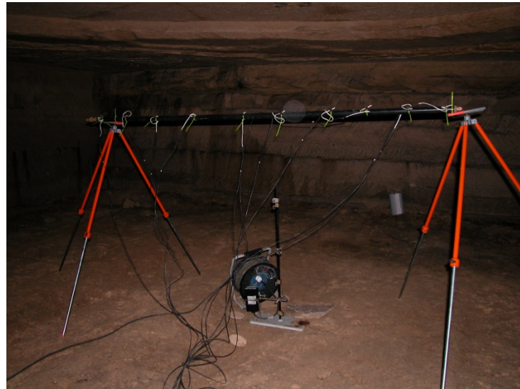
Figure 2: (a) Schematic cross-section of the experimental room S15 showing the four set-ups (AI, AII, AIII, and S) along with the positions of the temperature sensors (1-10 for each set-up); (b, c) photos of the set-up AIII in advance the heating experiments A2 and A4 (Table 1).
