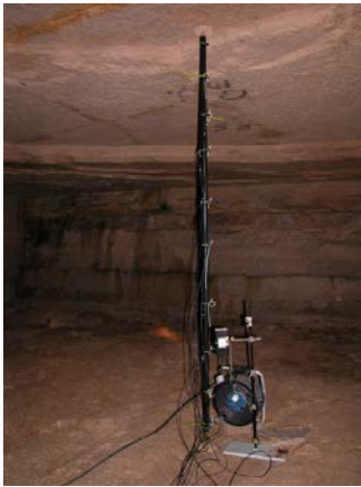
5 | Figure 2: (a) Schematic cross-section of the experimental room S15 showing the four set-ups (AI, AII, AIII, and S) along with the positions of the temperature sensors, (1-10 for each set-up); (b, c) photos of the set-up AIII in advance the heating experiments A2 and A4 (Table 1).
