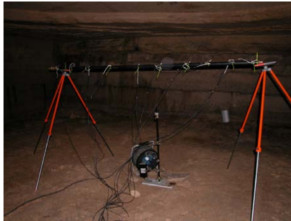
5 | Figure 2: (a) Schematic cross-section of the experimental room S15 showing the four set-ups (AI, AII, AIII, and S) along with the positions of the temperature sensors, (1-10 for each set-up); (b, c) photos of the set-up AIII in advance the heating experiments A2 and A4 (Table 1).
