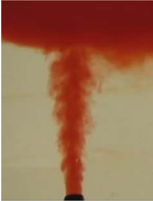
| Figure 16: A snapshot from a movie ( CarrozzoCarazzo et al., 2014, Supplementary Material S3 ), recording an experiment simulating a volcanic vent in a stratified water tank.
