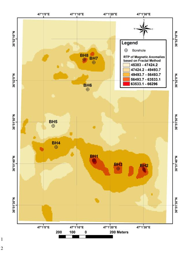
3 Figure 8. RTP map of Qoja-Kandi based on C-A method with drilled boreholes.
