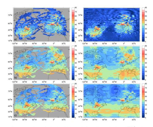
Figure 5. Reconstructions obtained at high resolution with masked out VTEC values where there is no ray coverage for: (a) spherical harmonics; (b) discrete Meyer; (c) Daubechies 4; and without the mask for (d) spherical harmonics; (e) discrete Meyer; (f) Daubechies 4. Values are in TECU (10<sup>16</sup> electrons m<sup>-2</sup>).
