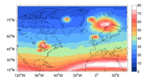
**Figure 2.** Simulated ionosphere with structures added to IRI2012. Values are in TECU (10<sup>16</sup> electrons m<sup>-2</sup>).
