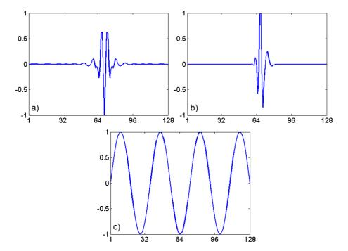
**Figure 1. (a)** Discretised Meyer basis function for a particular scale and translation; **(b)** Daubechies (4 tap) basis function with the same scale and translation as **(a)**; **(c)** a Fourier sinusoid component of the spherical harmonic basis functions. Basis functions are shown normalized to one and are interpolated for ease of viewing.
