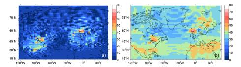
**Figure 9.** Reconstruction with **(a)** spherical harmonics and **(b)** discrete Meyer at high resolution with Gaussian noise added to the observations. The Gaussian noise has zero mean and a SD of 1 TEC unit.
