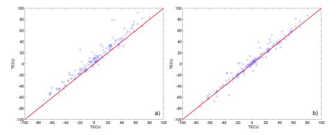
**Figure 6.** Scatter plot of the estimated offsets (y axis) vs. the true offsets (x axis) with (a) spherical harmonics and (b) discrete Meyer at low resolution.
