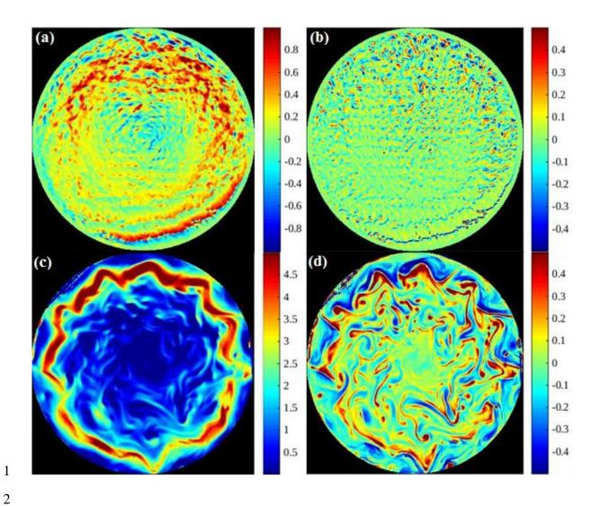
Figure 3. Flows generated by thermal forcing at t = 280 s (a, b) and by saline forcing at t = 150 s (c, d). Panels (a) and (c) show the x-component of velocity (azimuthal velocity) u while panels (b) and (d) show the dimensionless relative vorticity,  $\zeta/f_o$ . Salinity difference between the layers for the experiment with saline forcing (a, b) is S = 30 ppt. The center of the tank corresponds to the North Pole of the polar  $\beta$ -plane.
