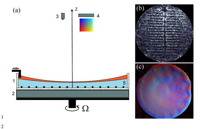
Figure 1. Sketch of the experimental setup (a) and view of the flow in the beginning of the experiments with the thermal (b) and saline (c) forcing: (1) cylindrical tank filled with water and installed on a table rotating with angular velocity  $\Omega$ ; (2) light box for the optical thickness measurements; (3) video camera; (4) light source with color mask; and (5) heating wire on the bottom.
