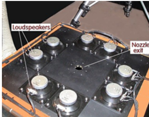
Figure 1: Photographic image of the acoustic excitation chamber with eight loudspeakers that are placed in flatwise manner to generate the necessary acoustic pressure in order to perturb the jet shear layer at the nozzle exit.
