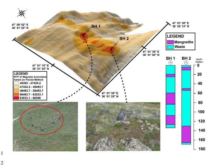
3 Figure 9. 3D RTP map of Qoja-Kandi based on C-A method with pictures from magnetite
