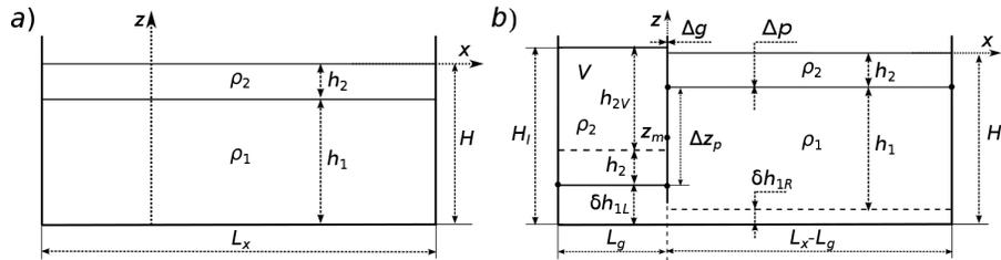
**Figure 1.** The geometry of the laboratory experiment **(a)** before and **(b)** after extracting the gate  $G$  and the volume of fluid  $V$ .
