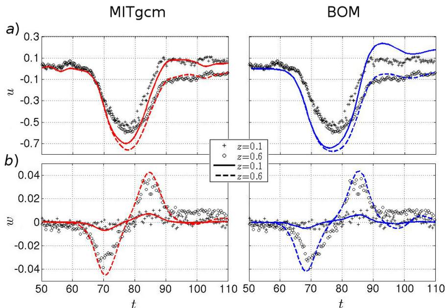
**Figure 6.** Horizontal **(a)** and vertical **(b)** near-bottom velocities at  $x = 0.66$ , measured in the laboratory experiment (symbols) and in numerical MITgcm and BOM models (lines) at a depth of  $z = 0.1$  (symbol “+” and the solid curve) and  $z = 0.6$  (symbol “o” and the dotted curve).
