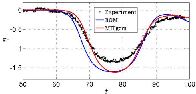
**Figure 5.** The comparison of the pycnocline displacement in the laboratory experiment and in the numerical MITgcm and BOM models: symbol “\*” – the data of laboratory measurements, solid red and blue curves – the results of the numerical simulations in the MITgcm and BOM models respectively.
